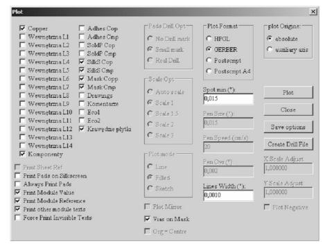
ATTENTION: The "Vision Mask" should be chosen only in case of boards that are not meant to be metallized; then the grommets won't be covered by soldiermask.
